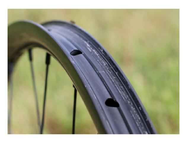
**Pl** Tiny 0.2mm tall ridges run around the circumference of the rim and are said to help hold a tire securely in place.
