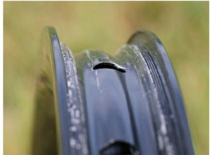
Spank says that the rim's 'W' cross section adds rigidity without adding grams. The rim bed isn't sealed, so you'll need to use the some tape and valve stems (not included) if you're going to run them tubeless.
